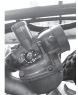
Idling speed adjusting screw
